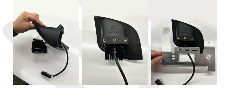
Insert the fog light into the housing and brackets
