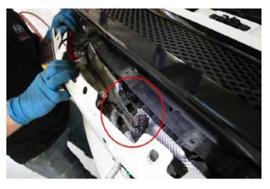
14. Remove antenna connector from left side of panel.
