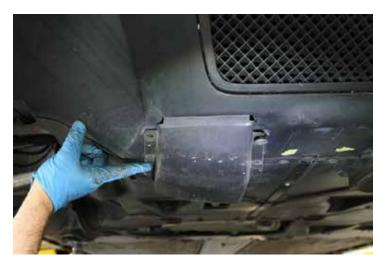
10. Remove (4) fasteners near the front center of the rear bumper diffuser panel.
