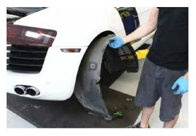
17. Remove (2) fasteners securing outer edge of heat shield to rear bumper on either side.
