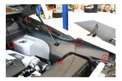
22. Using a small flathead screwdriver, carefully pry the engine cover strut off of the mount.
