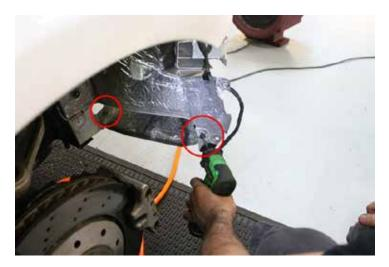
34. Remove (3) mounting screws from the bumper support.
