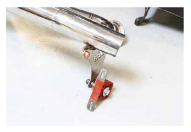
57. Re-assemble factory heat shield sections around Fabspeed x-pipe.
