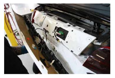
8. Remove (2) fasteners from the diffuser channel underneath both sides of the rear bumper assembly.
