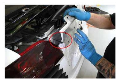
15. Remove all fasteners securing rear fender liners to the body/chassis.
