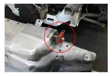
52. Remove snap-ring and slide spring and washer off of mounting post.
