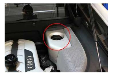
24. Carefully pry back trim panel and unplug the wires for the engine bay light.
