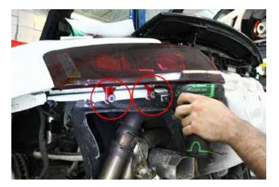
42. Remove hex nuts securing interior tail light mounting posts and remove tail lights.
