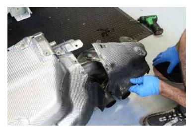
55. Remove front and back halves of heat shield.
