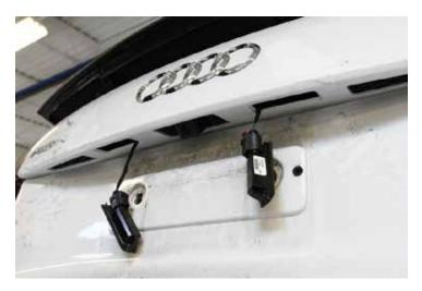
6. Locate and remove (2) additional fasteners located inside license plate light housings.
