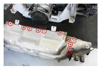
54. Remove side sections of heat shield.
