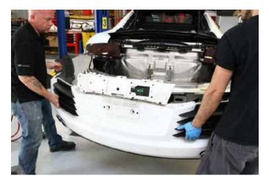
21. Remove fasteners securing passenger side engine bay trim panel.
