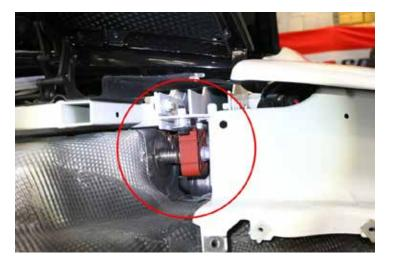
48. Remove v-band clamps from flex joints.
