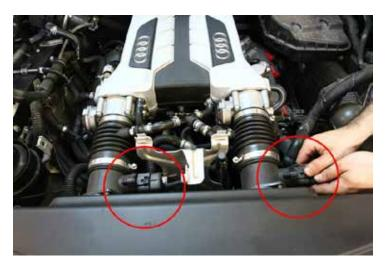
29. Loosen hose clamps enough to pull intake hoses off of the fittings.
