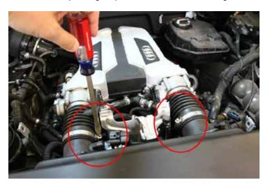
30. Remove the mounting screw from the bottom of each side of the airbox.
