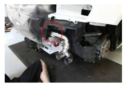
63. Test fit bumper and align Fabspeed tips so that they are positioned evenly against the integrated factory tips in the rear bumper.
