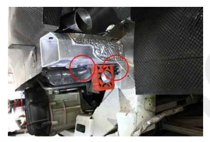
62. Attach the Fabspeed outlet tips to the slip-on elbow using the supplied v-band clamps, and slide onto Fabspeed x-pipe.
