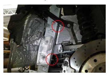
45. Remove the flanged hex nut located up inside the top of the heat shield, above the exhaust outlets.
