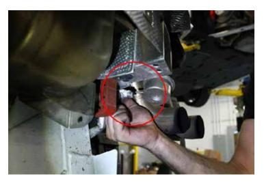
44. Remove the fasteners securing the vacuum line brackets and move vacuum lines out of the way.
