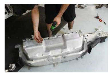
58. Place heat shield and x-pipe assembly back on vehicle and adjust fit.
