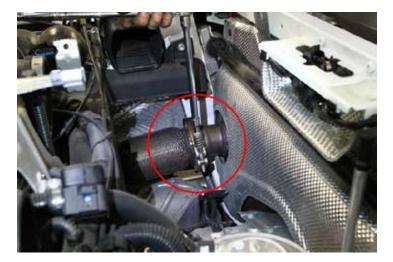
49. Remove fastener securing the heat shield inside of the rear wheel wells.
