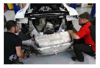
51. Remove retention bolt and muffler mount. (Save for re-use)
