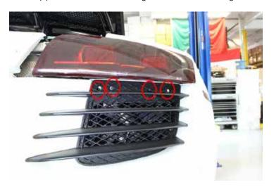
12. Remove fasteners securing rear upper trim panel.
