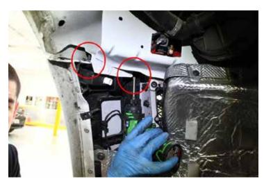
19. Gently separate rear bumper assembly and unplug wiring harness.
