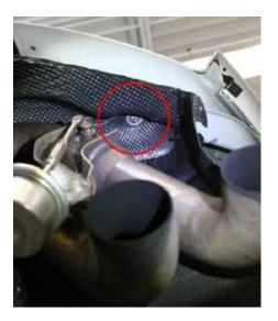
46. Remove lower muffler mounts.
