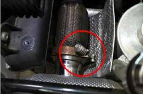
61. Re-fasten factory muffler mount back to the underside of the frame rail to further secure x-pipe.
