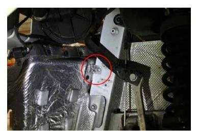
50. Remove muffler and heat shield assembly from the vehicle.
