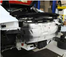
59. Re-fasten heat shield in the rear wheel wells.
