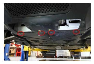
11. Remove (4) fasteners from behind the grilles beneath each tail light.
