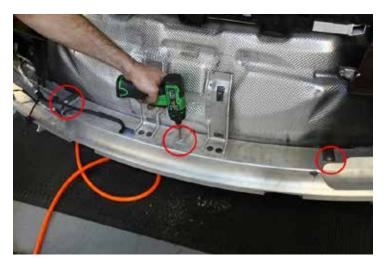
35. Remove the flanged hex nuts securing the outer lower heat shields to the bumper support.
