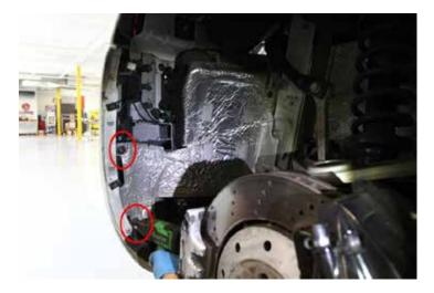
18. Locate and remove (2) fasteners securing the rear bumper to the upper body panel on either side.
