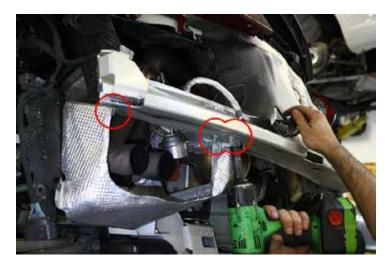
36. Remove flanged hex nut securing outer lower heat shield to frame/chassis and remove heat shield.
