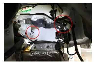
43. Unplug vacuum lines from muffler valves.
